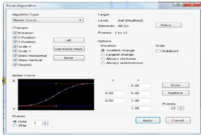
Top left is the Algorithm Type dropdown where you can chose for example Ease In/Out. Select the type of algorithm you want, and adjust the type accordingly then APPLY.
